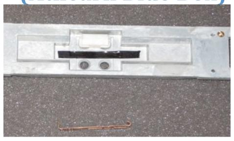
Next I removed the two tabs that are punched out of the brass that make contact with the frame. Connect a gray wire to this clip at the top front. To insure there is no possible short to the frame I installed a small piece of insulation before reinstalling the motor.
